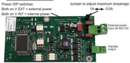
This option board does not require any software programming. It allows to add a minute, ½ minute, second or SR2-59 impulse output or TBT 24V DC 1A power supply. See page 35, the menu of the time outputs to set this output. Use the two Power DIP switches to select internal (24V) or external power (from 20 to 50 V).
