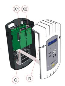
**RACK version :** Open the rack unit and install the option board(s) in the slots provided (X1) to (X2).
