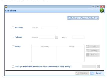
On this NTP Client screen, it is possible to choose the mode of reception of the time signal.
