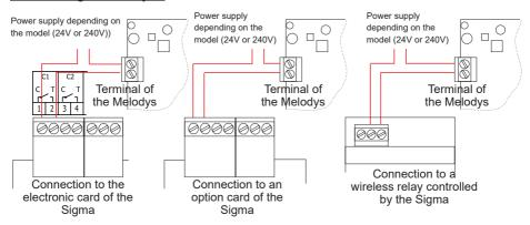
The Melodys can be connected directly to a relay output of the Sigma, an option card or a wireless relay.
