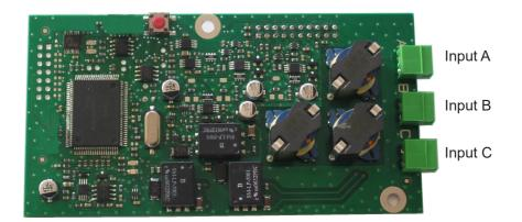
This card allows the addition of 3 external inputs.
