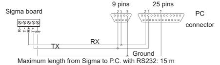
Synchronisation connection to a PC in RS422 Position of MA 45 PC interface DIP switches: Sigma board 00000 T+ T+ Interface 0000000000 00000000000 R-R+ MA 2 T-T+ 45 45 Link in RS422 Link in RS232 maximum length: 1200 m maximum length: 15m
