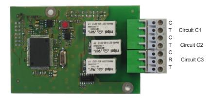
This option board does not require any software programming. It allows 3 relays to be added.
