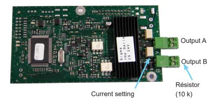
This option board does not require any programming. By default the time is the local time defined in the Sigma, with 1.2-second impulses, and the line is stopped.
