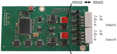
Output B programming DIP switches RS232 → RS422
