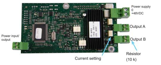
This option board does not require any programming. By default the time is the local time defined in the Sigma, with 1.2-second impulses, and the line is stopped.
