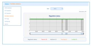
When the product starts up, the oscillator is in Freerun status (as if it had never been slaved). Then, it searches for the PPS signal to slave itself and switches to the Tracking status (tracking the PPS signal). Once it has been successfully slaved to the PPS, the oscillator locks on this signal (Locked status). If the PPS signal is lost, it switches to the Holdover status, then to the Freerun status when its own time zone is not longer reliable enough.
