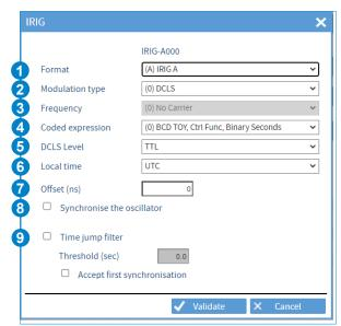
1 Choose the input format, according to the signal source: IRIG A/B/E/G, AFNOR 87500. The IRIG formats are defined by different pulse rates.
