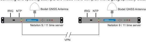
2 time servers installed on 2 different sites synchronise together (via NTP, PTP or IRIG) over a private network (VPN) This option assumes that the 2 Bodet time servers are in automatic mode (choice of the source) and have 3 independent synchronisation sources each.
