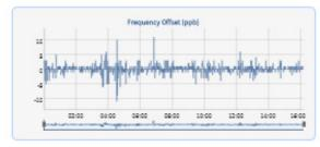
Correction applied to the oscillator
