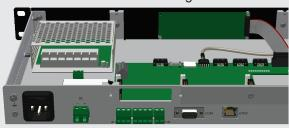
5) Place the option card by making sure that the outputs of the option card are aligned with the opening:
