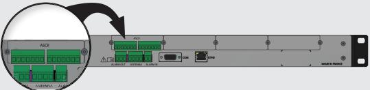
> Connectors: Removable 7-pin terminal block (pitch of 3.81 mm).
