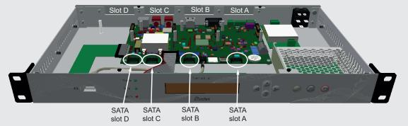
This operation applies to both Network option cards (RJ45 port) and Fibre Network option cards (SFP port). Make sure to connect the SATA cable to the right connector on the motherboard corresponding to the slot where the option card is installed.
