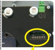
DIP switch Beware: in DHF version the DIP switch 2 must be in the ON position.
