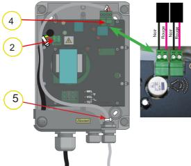
As the device is a class II device, there is no earth connection.
