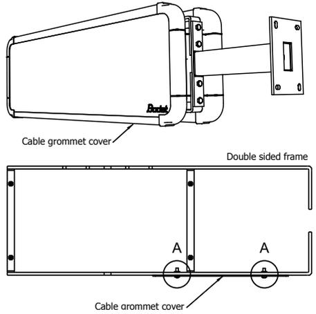
2/ Attach the cover of the bracket on the side of the double face support (only with vertical bracket) with the two 5 mm screws (detail B) (see single face assembly 4/).
