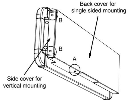
3/ Tighten the 4 screws in contact with the vert. bracket single face cover and then lock the 4 nuts on the double face support.
