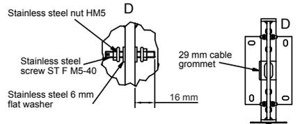
3/ Place the 4 screws (D) at 16 mm. Do not fit the nuts and washers.
