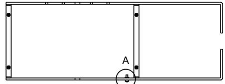
5/ Attach the bracket to the wall with the two 8 mm (HMT Led 10) or four 8 mm (HMT Led 15 and 20) or 10 mm (HMT Led 25) threaded rods plus chemical sealing (recommended).
