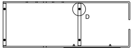
4/ Attach the bracket to the wall with the two 8 mm (HMT Led 10) or four 8 mm (HMT Led 15 and 20) or 10 mm (HMT Led 25) threaded rods plus chemical sealing (recommended).
