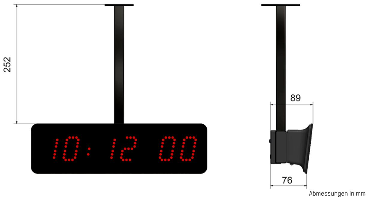
Abmessungen in mm
